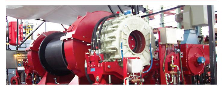
ADS drawworks are equipped with AC motors which provide significantly more performance and have made possible a machine that requires approximately half the space and weight with less maintenance than traditional drawworks.
