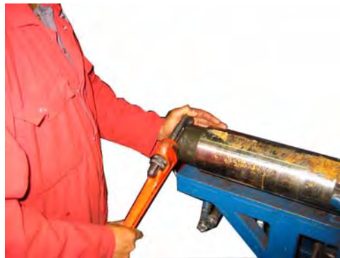
Use a wrench to fit the end cap
