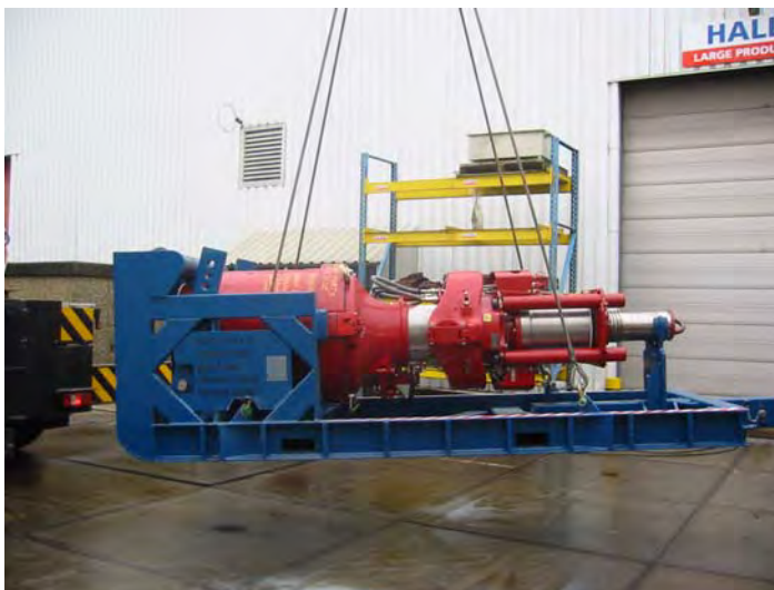
Lifting horizontally (with or without CRT)
