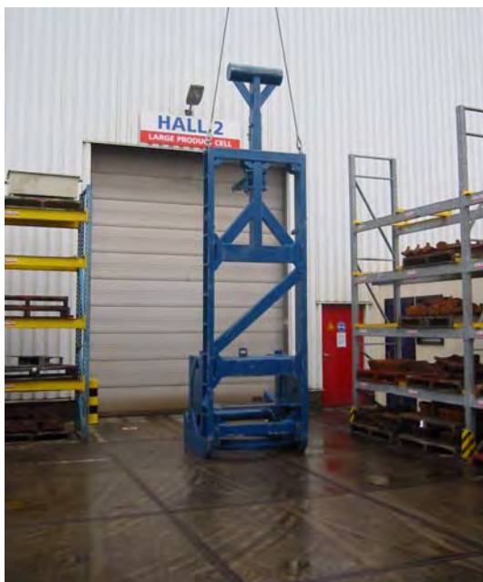
Lifting the skid vertically (Do NOT lift like this with CRT in skid)
