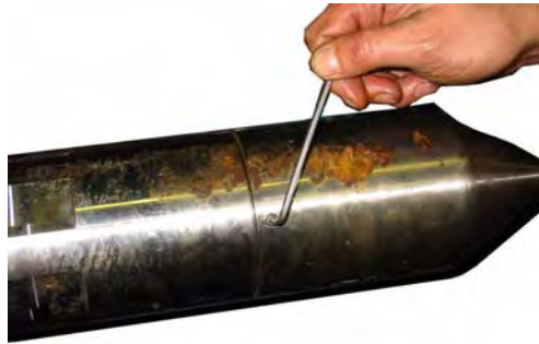
Finally secure the hexon screws
