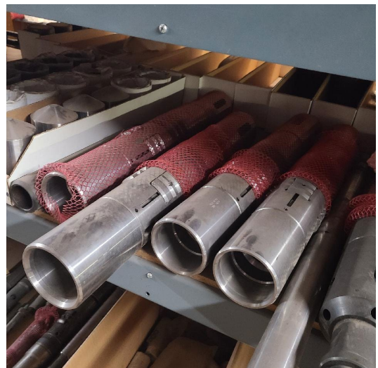
Inconel Tools: (6) 3.81 R Lock plugs and (2) R Running Tools
