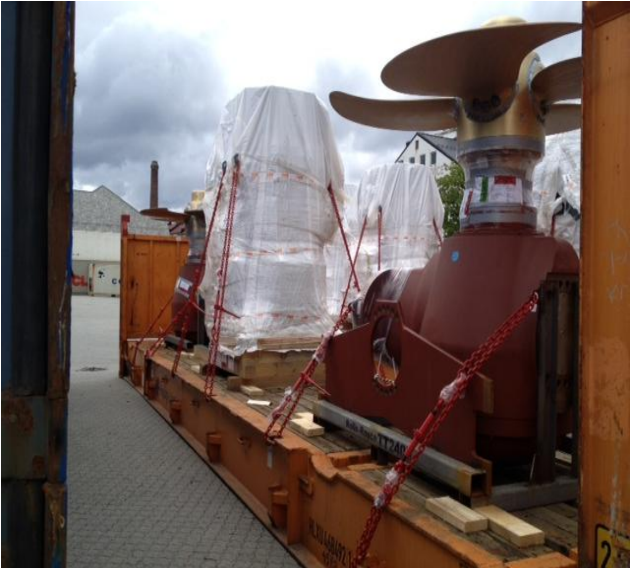
Picture 2 depicts the 2 x tunnel thrusters, TT2400.
