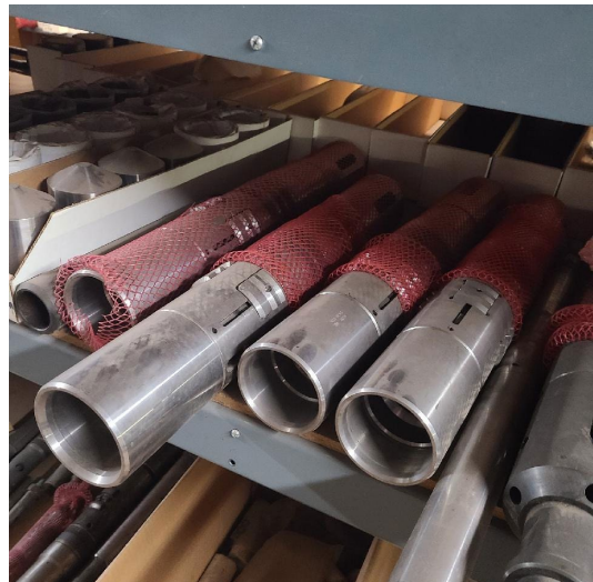
Inconel Tools: (6) 3.81 R Lock plugs and (2) R Running Tools
