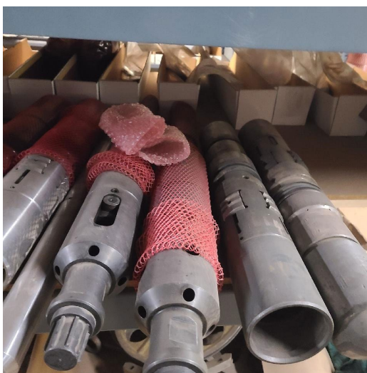
Inconel Tools: (6) 3.81 R Lock plugs and (2) R Running Tools
